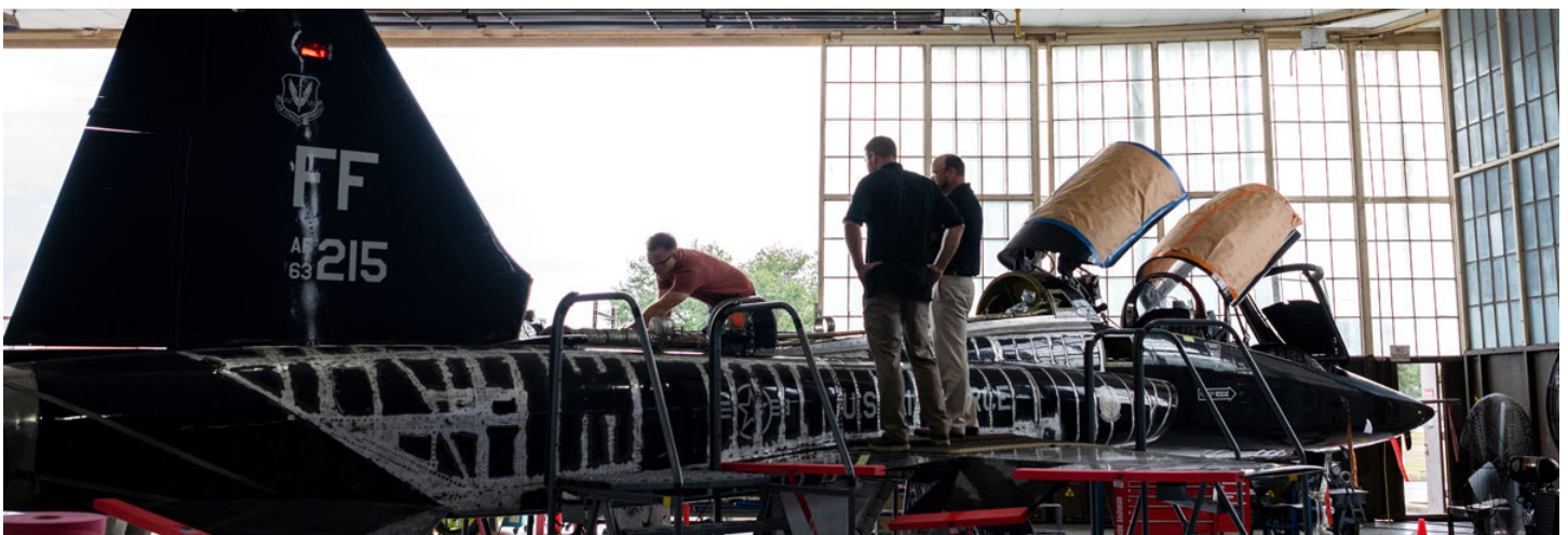
Zach Burleson (left), 809 th Aircraft Maintenance Squadron, Non-Destructive Inspection technician, works on a T-38 as part of the Talon Repair Inspections and Maintenance (TRIM) program as Larry Hall (center), 809AMXS, and Robert Pilarczyk (right), Hill Engineering observe at Joint Base San Antonio-Randolph, TX. The TRIM program will be performed on 190 T-38 aircraft. The capability allows for localized depot-level maintenance to replace or repair key parts.
